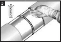
Ensure that the mainline coating edges are beveled to 30°. If there is the presence of oil, grease, or other surface contaminants; clean the exposed steel and adjacent pipe coating with a solvent cleanser.
