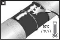
Pre-heat the epoxy and the abraded coating to 90°C +/-5° (195°F +/- 10°) with the appropriate propane torch. This will substantially cure the epoxy and ensure proper flow and bonding of the sleeve adhesive. **Do not use an intense flame on the mainline coating.** If a film develops on the mainline coating because of preheat, use a surface abrasion tool to remove it.
