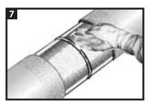
Wipe clean or air blast the steel and coated areas to remove foreign materials.
